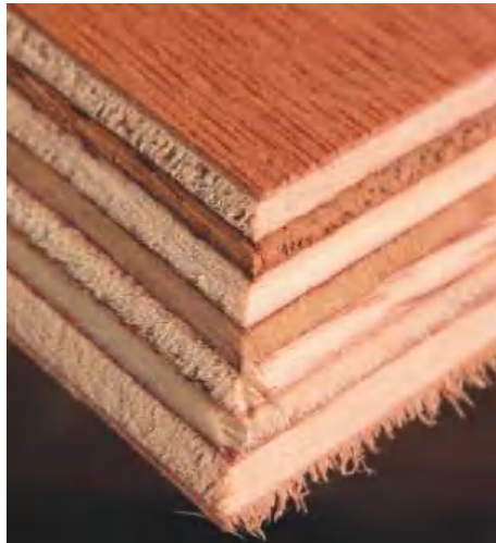
▲ Pic.18 Plywood has grain in both directions, making large panels less liable to distortion
